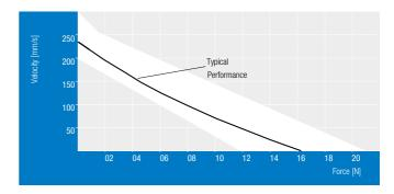
In case of use in Z-direction the motor characteristics speed/force must be taken into consideration
